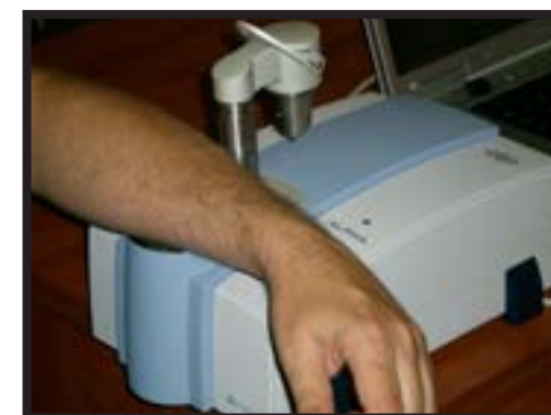
Sunscreen deposition being measured on an arm by ATR-FTIR.
